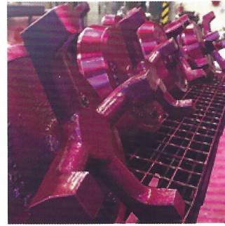
LIQUID PENETRANT INSPECTION
